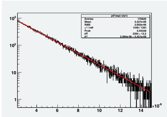
**Figure 1.** Typical time spectrum of delayed-timing charged particles observed at the exit of D-line. The origin of horizontal axis is a time of the 1st proton pulse. In order to protect the counter from the prompt burst, signal at around the proton pulses are masked.
