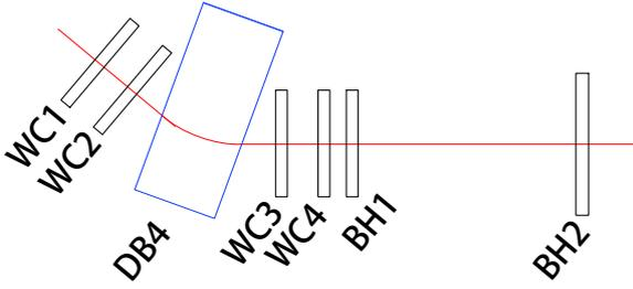
**Figure 3.** Schematic layout of the electron spectrometer.
