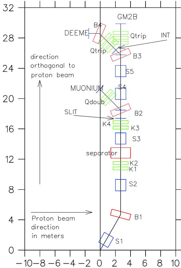
**Figure 2.** Layout of the new beamline for DeeMe (DEEME), surface muon (MUSR) and muon  $g - 2$  (GM2B) experiments. S1–5 are solenoids, B1–4 are dipole bends, K1–4 are kicker magnets, Qdoub and Qtrip are quadrupole- doublet and triplet, respectively.
