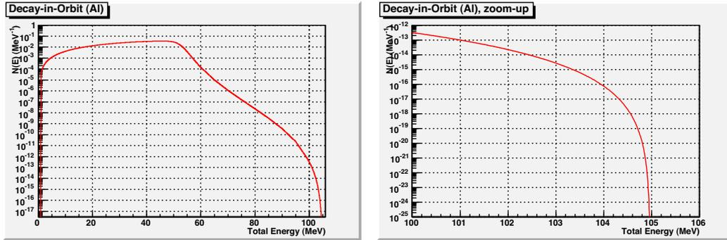
Figure 1: Total energy spectrum of electrons from muon decays in orbit for Aluminum.
