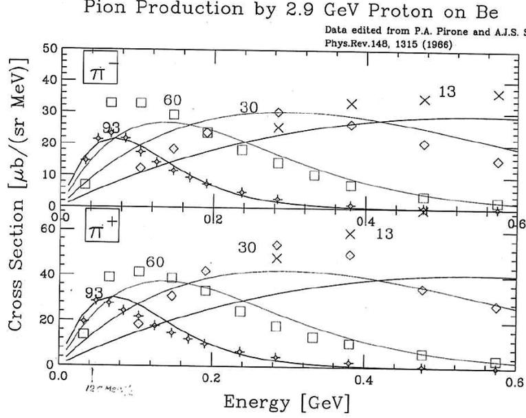
Figure 4: Pion production cross section by 2.9 GeV proton on Be target.
