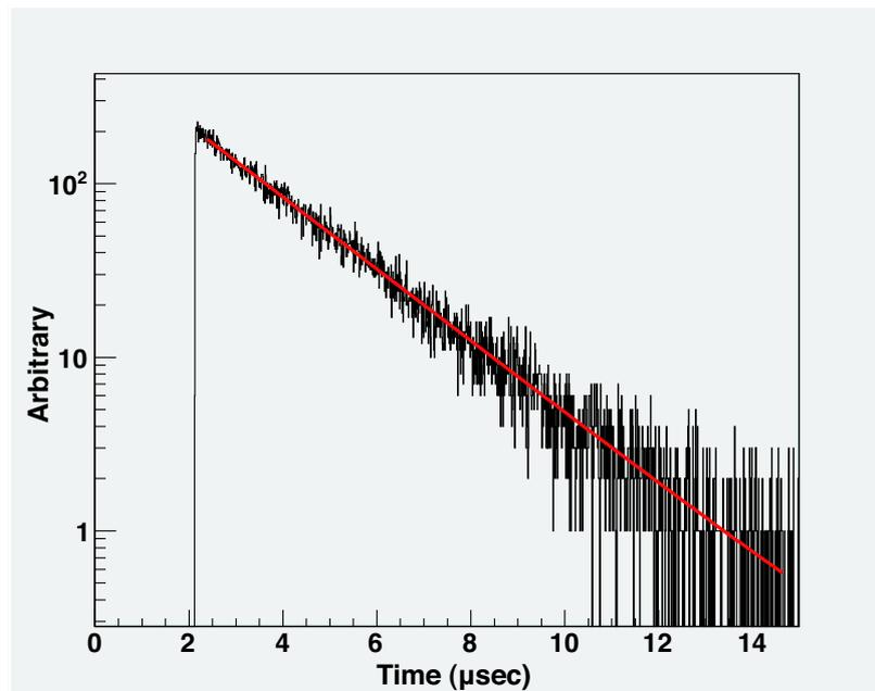
Figure 5: Typical time spectrum observed at the exit of D2 beamline. The origin of horizontal axis is a time of the 1st proton pulse.
