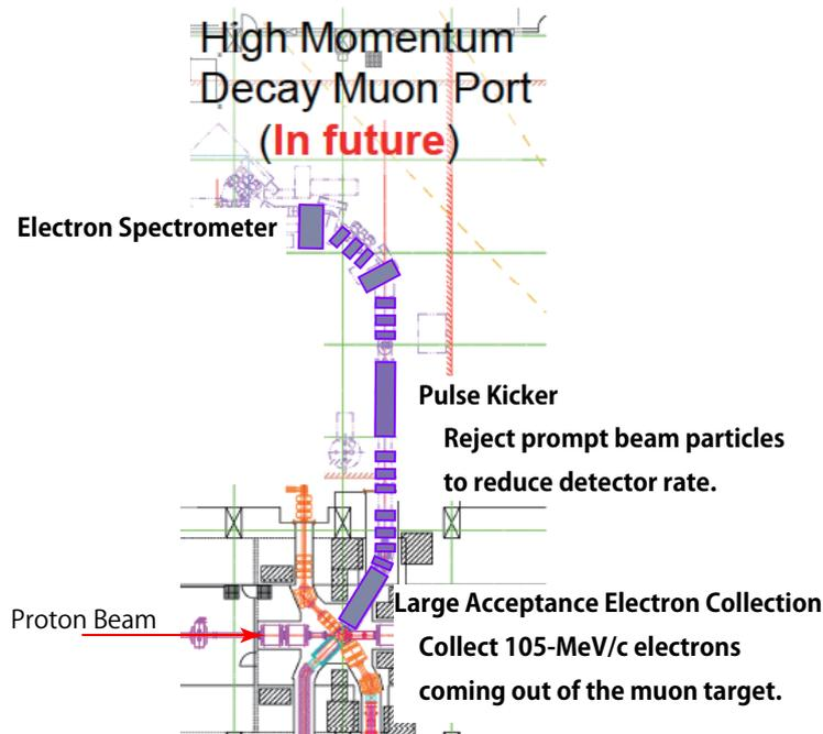
Figure 2: Schematic plan of the Configuration-A with the new beamline placed at the High Momentum Decay Muon Port.
