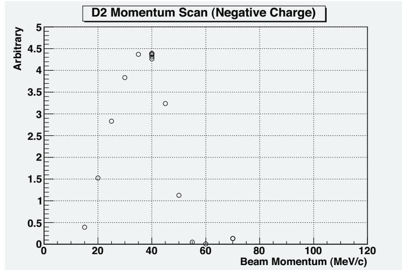
Figure 6: Momentum spectrum of the beam electron obtained by scanning the momentum setting of the beamline. A 6-mm<sup>t</sup> Lead absorber was placed in front of counters to absorb beam muons.
