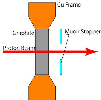
Figure 3: One example of how the Aluminum muon stopper could be installed near the muon target. Please note that the design is not final.
